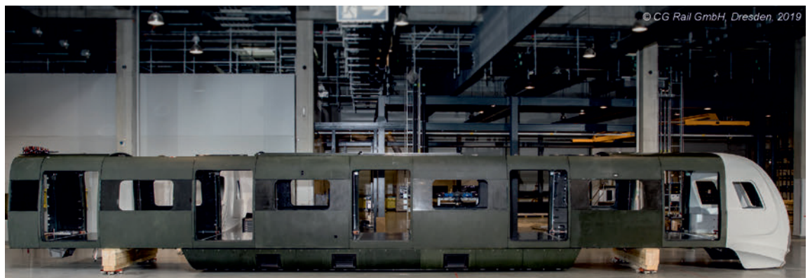
Figure 6: Lightweight car body made of CFRP
